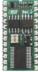
Figure 1-2 BASIC Stamp 2 Microcontroller Module
