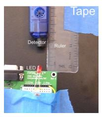
To determine the relationship between the observed brightness of a light source and the distance from the source.
