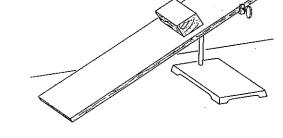
Conclusion: The coefficient of sliding friction was found to be ... by the inclined plane method.
