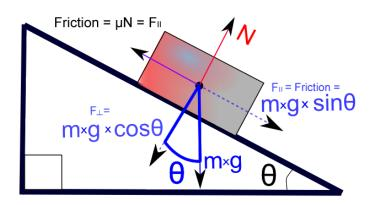
The purpose of this lab is to measure the coefficient of static friction between two surfaces. Let's use the physics textbook and a quarter.
