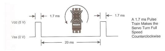
Those are the extremes. A pulse width of 1500 ms causes the servo to stay still, assuming it has been calibrated properly. If not, you can calibrate it by gently adjusting the potentiometer using a small screwdriver.
