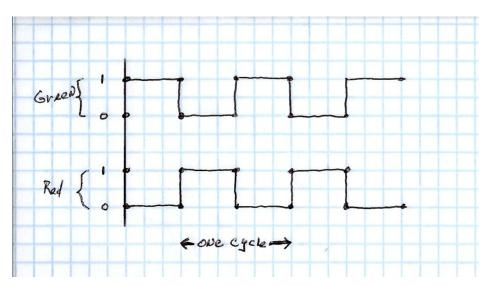
Consider time along the X axis. You can see that when the green light is on (1), the red light is off (0), and vice-versa. The length of one cycle is not given. In real life that would be several seconds. However, for the sake of keeping your debugging time reasonable, we will make the time of one cycle 4 seconds. It should be obvious that the cycle time would be easy to adjust when we go from the lab to the real world.
