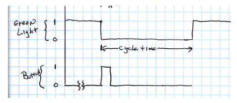
Explanation: The light remains green until the button is pushed. The length of time you hold the button does not matter. Once the button is pushed the green light goes off and stays off for the cycle time. We will make the cycle time 20 seconds. After 20 seconds has passed the green light comes back on.
