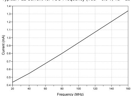
Typical PLL Current vs. VCO Frequency (Vdd = 3.3 V, Ta = 25° C)
