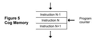
In Stage 1, instruction N, pointed to by the Program Counter, is fetched from cog memory during clock cycle M. During cycle M+1 the result from the previous instruction is written to memory. The reason the previous instruction result is written after the current instruction is fetched will be explained shortly.
