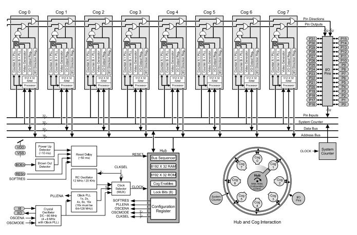
Figure 1: Propeller P8X32A Block Diagram
